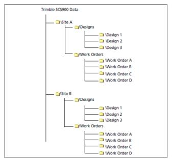
Information on a controller is arranged in the following levels:
