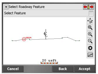
If the node is on the finished grade model, the name of the node would be SHLD, for example. If the node being selected is on the subgrade adjusted surface, it would be named SHLD-0.250; meaning it is the SHLD node, but it has a -0.250 m. A subgrade can be entered by accessing Road Settings through the Trimble icon menu while in Road Stakeout mode.
