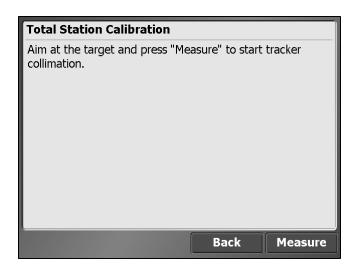
**Note** – There can be two reasons for significant change between old and new values: The total station has received a knock or bump in transit that may need a service correction. There has been an observation error.
