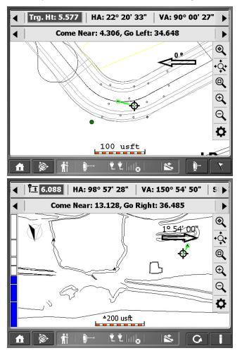
manually turn the total station until reaching the direction of the stakeout point.
