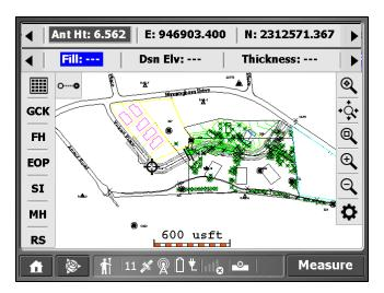
If the software is not automatically connecting to your positioning device, go to the *Home* menu and tap GPS or Total Station to start the setup.
