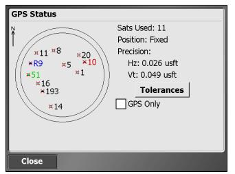
The **Tolerances** button, which appears when the controller is connected to an SPS receiver, is a shortcut to the RTK Precision option. The *GPS Only* check box enables you to toggle between using GPS and GNSS.
