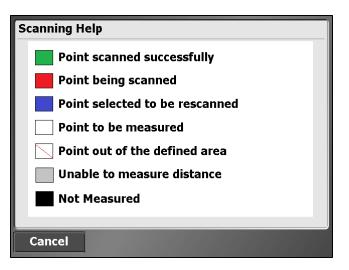
To rescan any cells, tap OK to return to the measured cells display. Tap the associated grid sectors with your stylus. Selected sectors turn blue. Once the selection is made, tap Rescan. Repeat the rescan function until results are satisfactory and then tap Finish.
