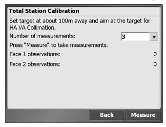
The collimation test computes the collimation error, stores the error inside the total station and then corrects all subsequent measurements for that error before displaying them on the screen or storing them in memory.
