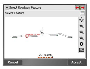
If you are navigating up station, the normal cross section view is displayed left to right as expected. If however, you are navigating down station, then the cross section would normally be back to front. To reverse the view of the section, make sure Road Stakeout mode is selected, then select the Trimble icon menu / Road Settings, and change the view setting to up station or down station.
