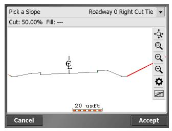
In the top line of the display, the roadway that the tie slope is associated with is displayed. In the example above, there is only one roadway in the selected road job, and that was not named—hence Roadway 0 is displayed.
