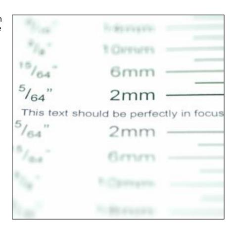
If the part of your pic that's in focus is so far back that the focus line is way out of focus then you have a problem with back focus, as in this example.
