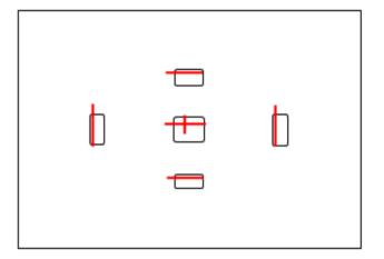
Think of each of those red lines, or AF sensors, as tiny digital cameras, except, instead of being a rectangle filled with rows and columns of pixels, as a normal camera would be, they're each just a row or column – a line of pixels.
