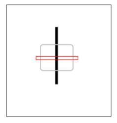
The focus sensor is positioned so that it can "see" the black line on our test page.
