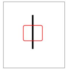
This is because the camera's AF system is easily able see a point of contrast and to adjust the focus until this contrast is maximised for best focus.
